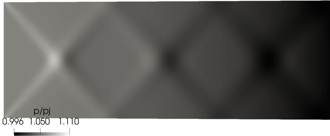
FIGURE 5.22 – Pressure contours for the final nozzle design, cfg15 .
