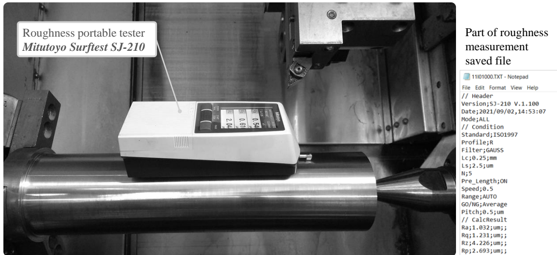
Figure 37. Mitutoyo portable roughness tester model Surftest SJ-210 . Measurement setup (left) and result example (right).
